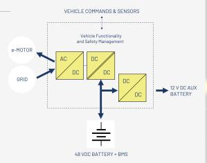
10 kW Galvanically Insulated Bidirectional DC/DC Converter
