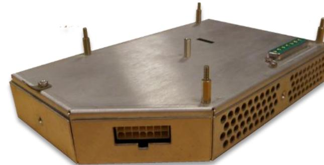
*Two units to generate the low voltages but with high current ratings close to the consumer and to provide filters and linear regulations for low-noise supply voltages for the analog section of the front end*
